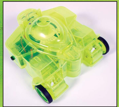
FIGURE 28. A program disk installed in Binary Player Robot. Please note the speed shift levers on the rear of each motor gearbox.
